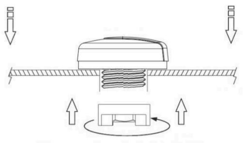
Recommended torque for Mounting is 3.92N·m Maximum torque for Mounting is 4.9N·m
